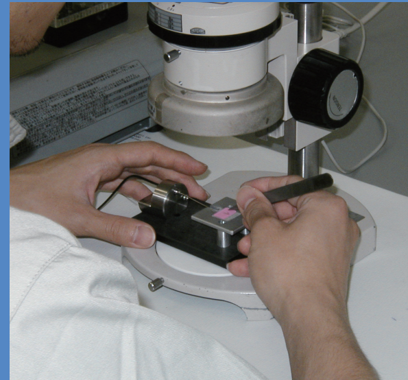
Kono Seisakusho's veteran machinists craft ultrafine needles just 30 micrometers in diameter and 800 micrometers long by hand
